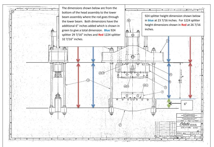
3. On 1624 splitters dimension check from the bottom of the head to the top surface of the lower beam assembly is set at 31 .13" inches If you are checking these dimensions from where the tie rod enters the head assembly and to the bottom beam assembly same you need to add an additional (6") inches which will give you an overall dimension of 37 .13" inches. (Please see print and dimensions below
